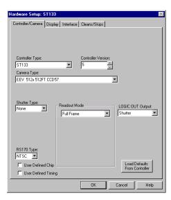
Figure 4. WinView/32 Controller/Camera Setup Tab Page
